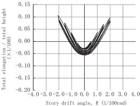
Figure 9. Relationship between axial elongation of columns and story drift.
