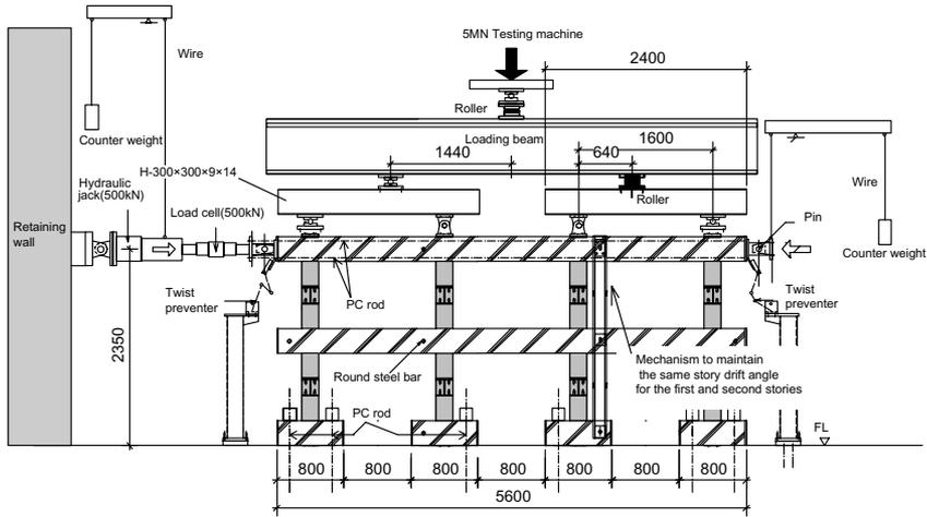
Figure 5. Loading set-up.
