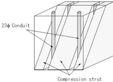
Figure 13. Ineffective width due to conduits.
