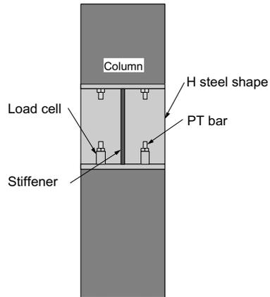
Figure 4. Column-to-column connecting device.
