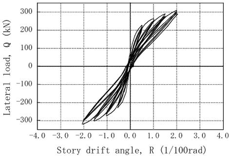
Figure 8. Experimental cyclic lateral load-drift behavior.
