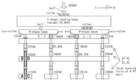
Figure 6. Axial force in each column.
