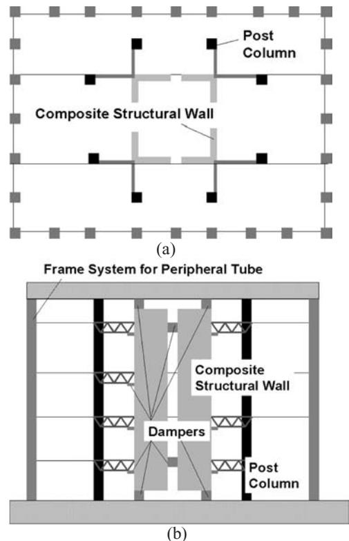
Figure 1. Prototype building: (a) plan; and (b) section.
