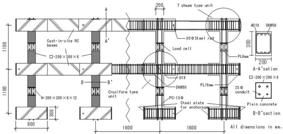
Figure 2. Self-centering frame system studied.
