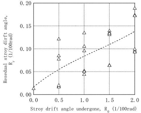
Figure 10. Relationship between residual story drift and story drift undergone.
