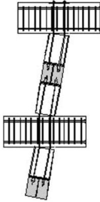
Figure 3. Schematic deformed configuration of unbonded PT precast column.
