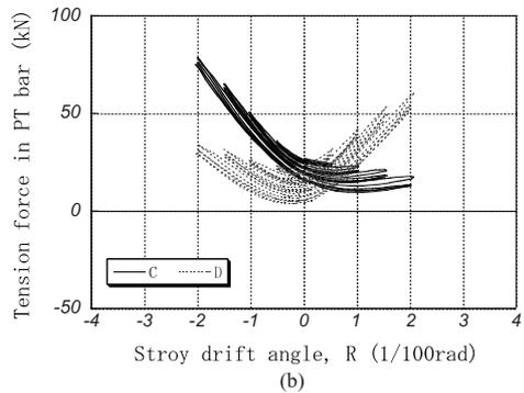
Figure 11. Tension force-drift behavior of PT bars: (a) PT-A, B; and (b) PT-C, D.
