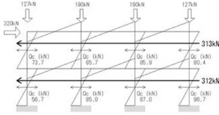
Figure 12. External load and internal force in the frame at the ultimate state.
