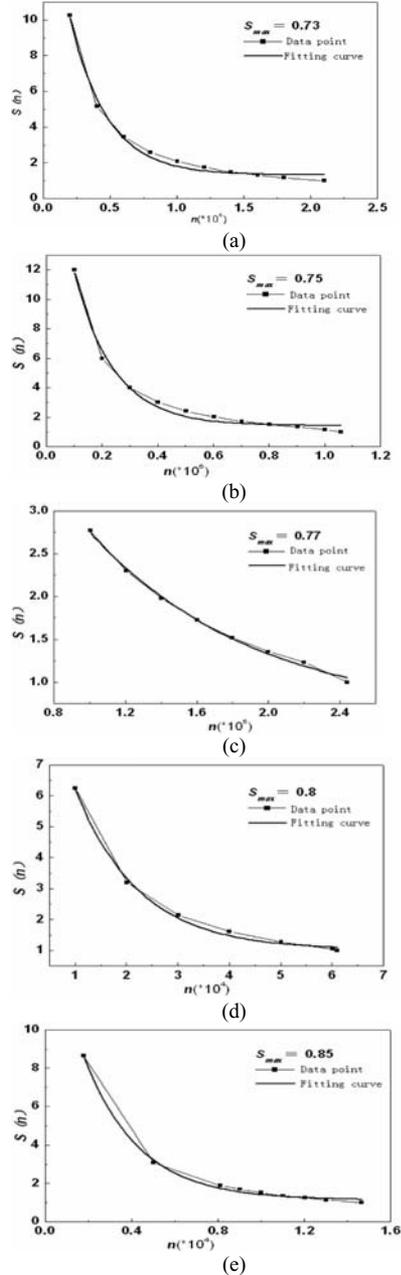
Figure 3.  $s_i(n_i) \sim n_i$  curves under constant-amplitude cyclic loads at five stress levels.
