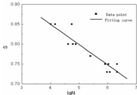
Figure 6.  $S - \lg N$  data points from the high frequency fatigue tests and the corresponding fitting curves.
