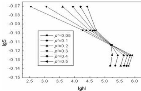
Figure 7.  $\lg S \sim \lg N$  fatigue curves corresponding to different failure probabilities.
