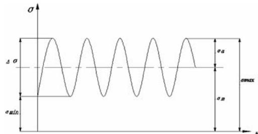
Figure 1. Relationship between fatigue load parameters.
