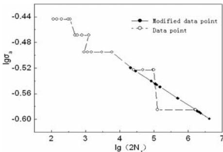
Figure 5.  $\lg \sigma_a \sim \lg(2N_f)$  curves obtained from modified curves of high-frequency fatigue tests and low-frequency fatigue tests.
