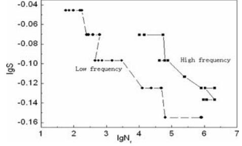
Figure 4.  $\lg S \sim \lg N_f$  curves under high-frequency and low-frequency fatigue loads.
