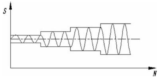
Figure 2. The loading form of stepping-amplitude cyclic loading tests.
