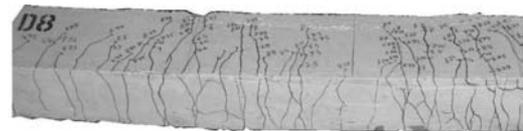
Figure 6. Cracks at bottom and side of beam D8 at failure.
