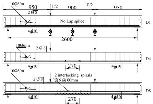
Figure 2. Details of some tested specimens.
