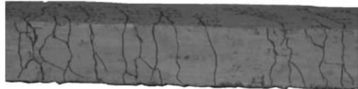
Figure 5. Crack pattern at the bottom of beam D5 at failure.
