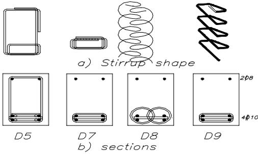
Figure 3. Details of transverse reinforcement.
