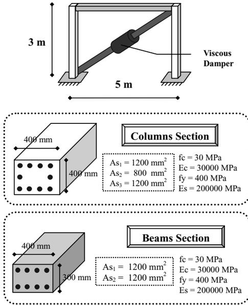
Figure 4. Single storey frame example and sections properties.
