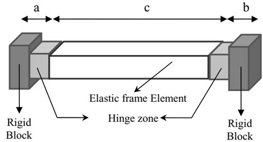
Figure 2. Inelastic modeling of frame member.
