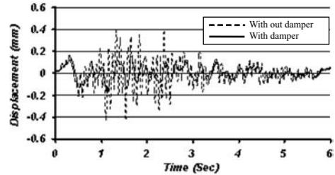
Figure 7. Displacement of top node of single story model in X direction ( $\bar{C}_d = 1300$ ).
