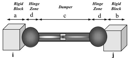
Figure 3. Three dimensional damper element with two plastic hinges at ends.
