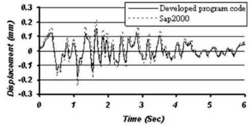
Figure 6. Comparing the results of developed finite element program code and SAP2000 software (displacements of top node in X direction).
