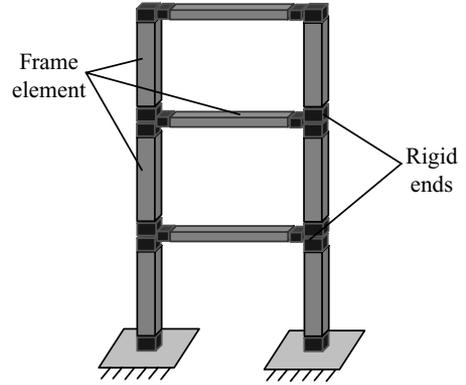
Figure 1. Mathematical model of building structure.
