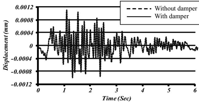
Figure 8. Displacement of top node of single story model in Y direction ( $\bar{C}_d = 1300$ ).
