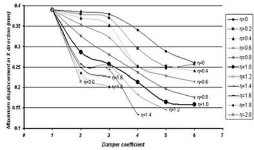
Figure 9. Comparison top node displacement of single story example in X direction with various damper velocity exponential coefficients ( $\eta$ ) and damping coefficient ( $\bar{C}_d$ ).
