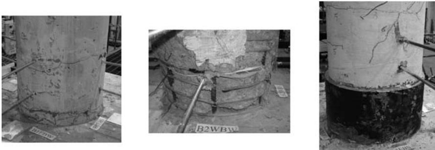
Figure 6. Lower plastic hinge after final motion: left to right, SMA pier, PT pier, and ISO pier.
