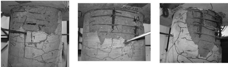
Figure 5. Upper plastic hinge after final motion: left to right, SMA pier, PT pier, and ISO pier.
