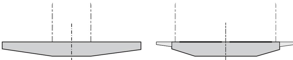
**Figure 0.11** Systems with two vertical cable planes positioned between three separate traffic lanes
