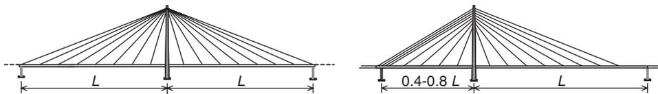
**Figure 0.6** Two-span cable stayed bridges
