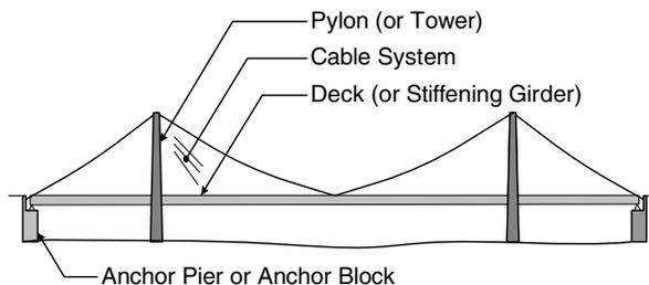
**Figure 0.1** Main components of a cable supported bridge
