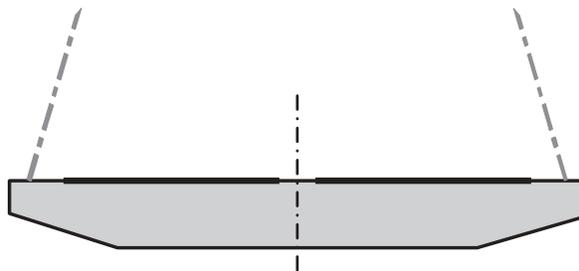
**Figure 0.14** System with two inclined cable planes
