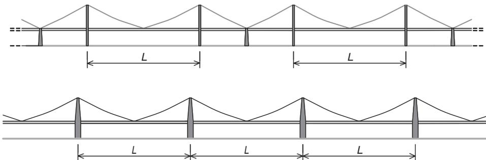
**Figure 0.7** Multi-span cable supported bridges
