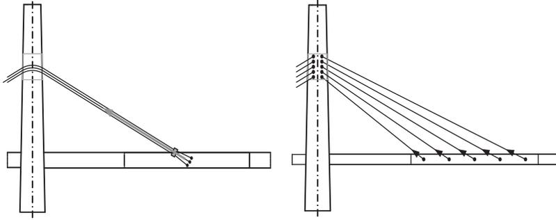
**Figure 0.8** Cable stayed system with few multi-strand cables (left) and a multi-cable system (right)
