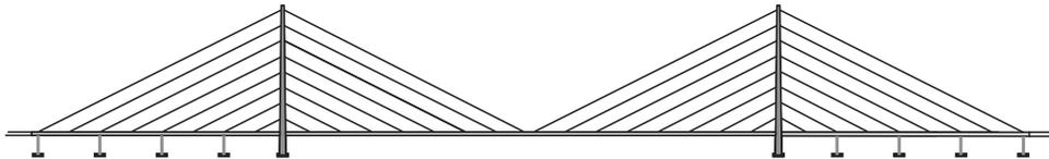
**Figure 0.5** Harp system with intermediate supports in the side spans
