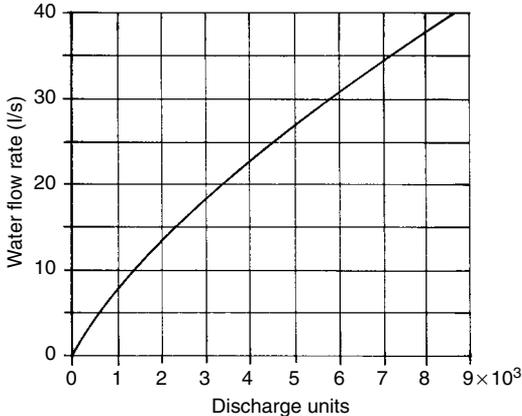
9.4 Simultaneous flow data for foul- and surface-water drains (reproduced from data in *CIBSE Guide* (CIBSE, 1986) by permission of the Chartered Institution of Building Services Engineers).
