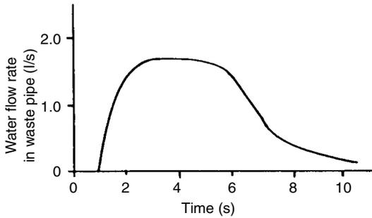
7.1 Discharge of water from a sanitary appliance.
