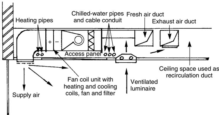
5.14 Fan coil unit installation in a false ceiling.
