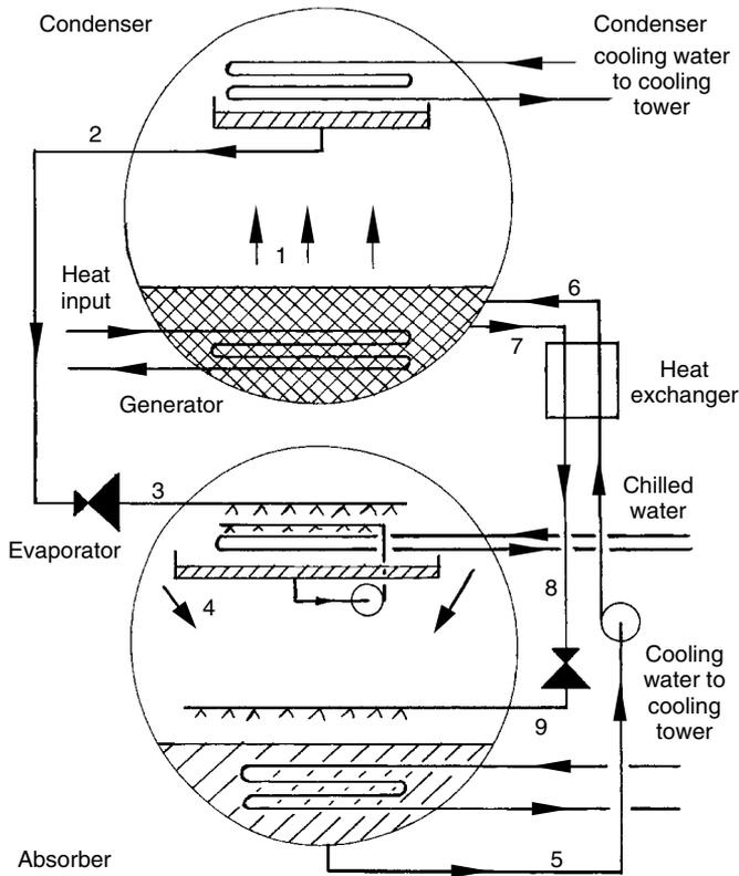
5.19 Two-drum absorption refrigeration cycle.
