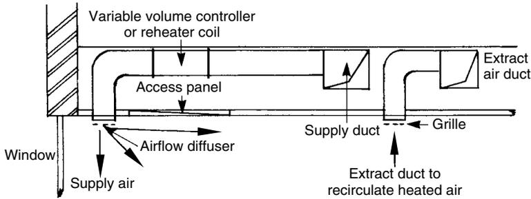
5.11 Single-duct all-air installation in a false ceiling.
