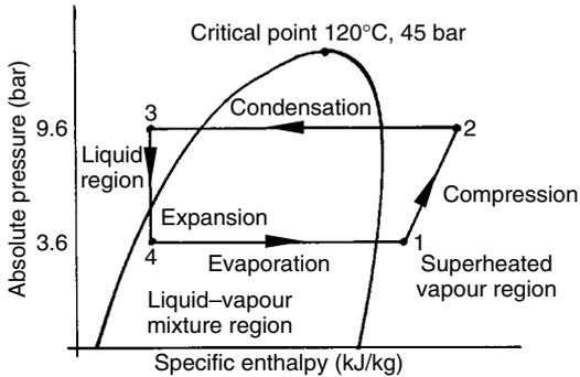
5.17 Pressure–enthalpy diagram for a refrigerant showing the vapour-compression cycle.
