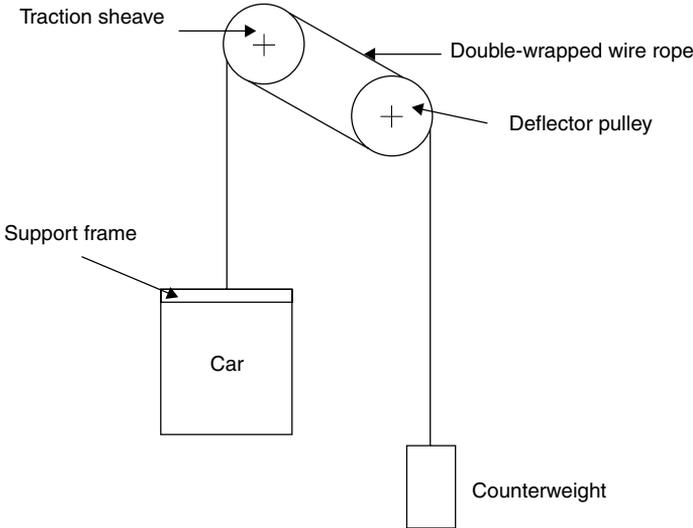
17.2 Traction arrangement for a high-speed passenger lift.
