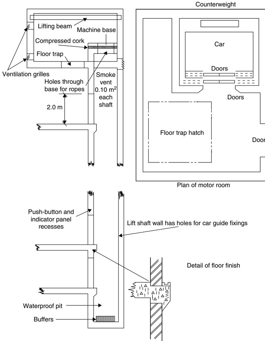
17.5 Constructional features of a passenger lift shaft.
