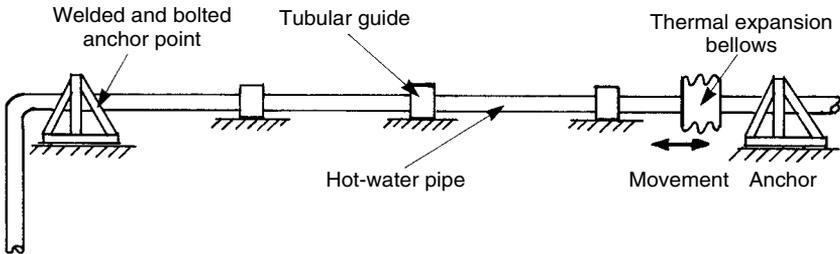
16.10 Complete pipework installation for thermal expansion provision.
