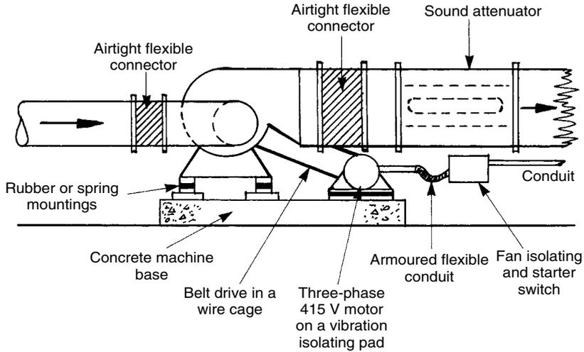
16.14 Flexible connections to an air-conditioning fan.
