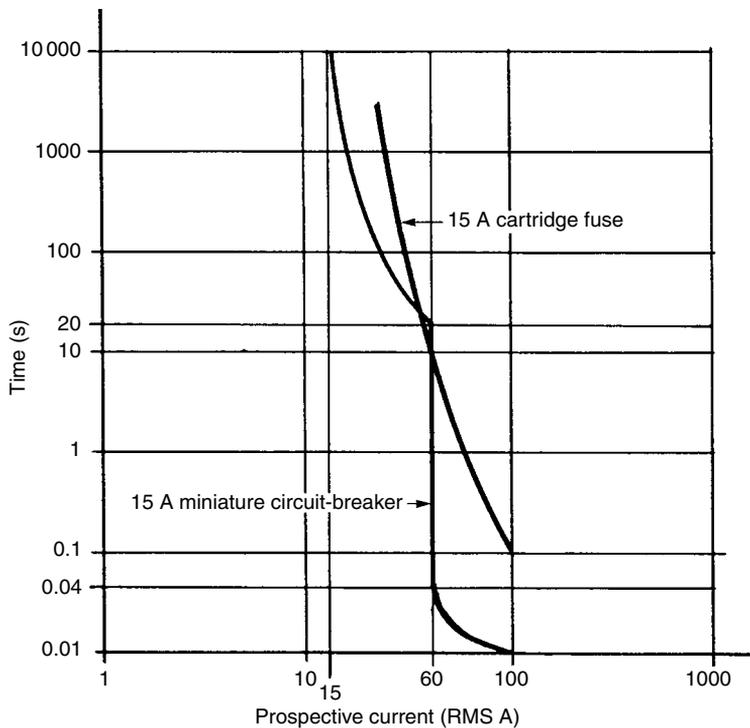
13.8 Time–current characteristics of a cartridge fuse and a miniature circuit-breaker.
