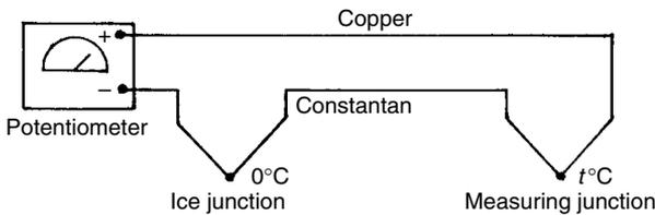
1.9 Basic thermocouple circuit and calibration graph.
