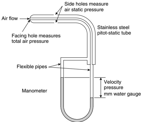
1.8 Pitot-static tube and U-tube manometer.
