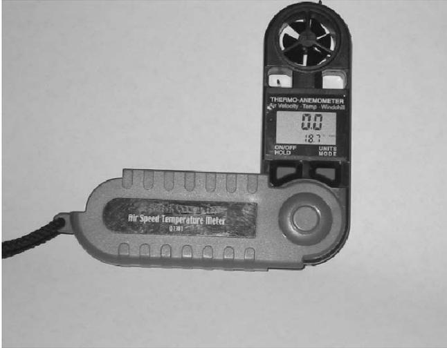
1.7 Thermistor anemometer.
