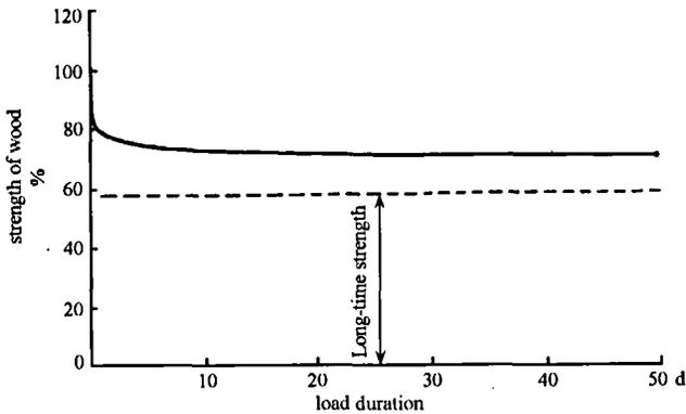
Figure 9.6 The Creep Rupture Strength of Wood
