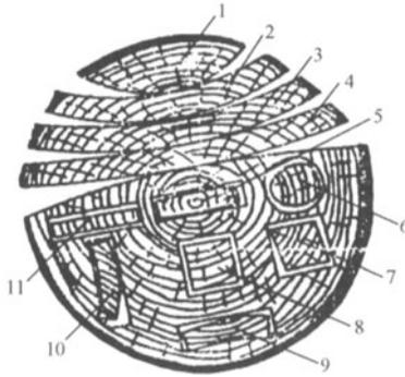
Figure 9.4 Deformation of Wood's Section Shape after Drying
