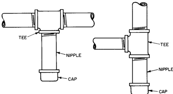
FIGURE 14.13 Drips for gas piping.
