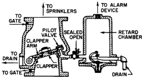
FIGURE 14.15 Alarm-check valve.
