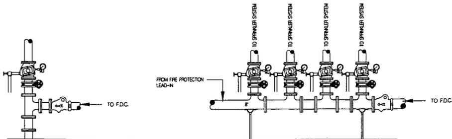
FIGURE 14.19 Single riser (left), manifold system with multiple risers (right).
