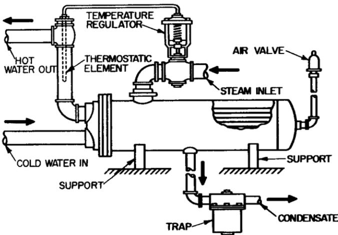
FIGURE 14.8 Instantaneous heater for domestic hot water.
