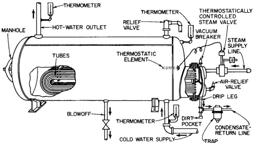
FIGURE 14.7 Storage heater for domestic hot water.
