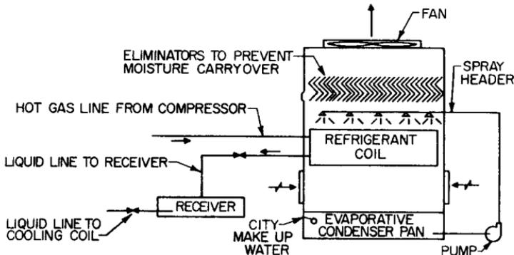
**FIGURE 13.32** Evaporative condenser for an air-conditioning system.
