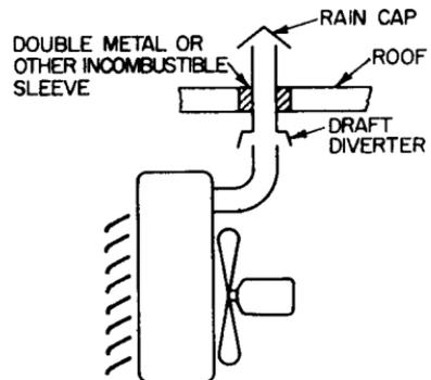
FIGURE 13.18 Connections to outside for gas-fired unit heater.
