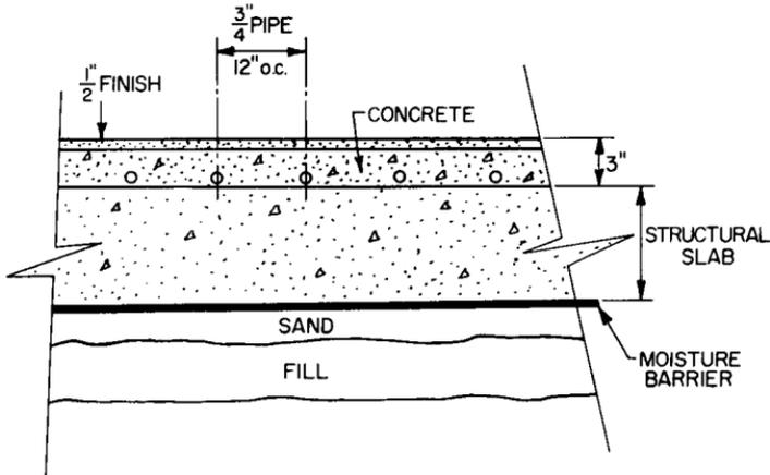
**FIGURE 13.27** Pipe coil embedded in a concrete slab for outdoor snow melting.
