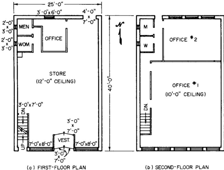
FIGURE 13.3 First-floor and second-floor plans of a two-story building.
