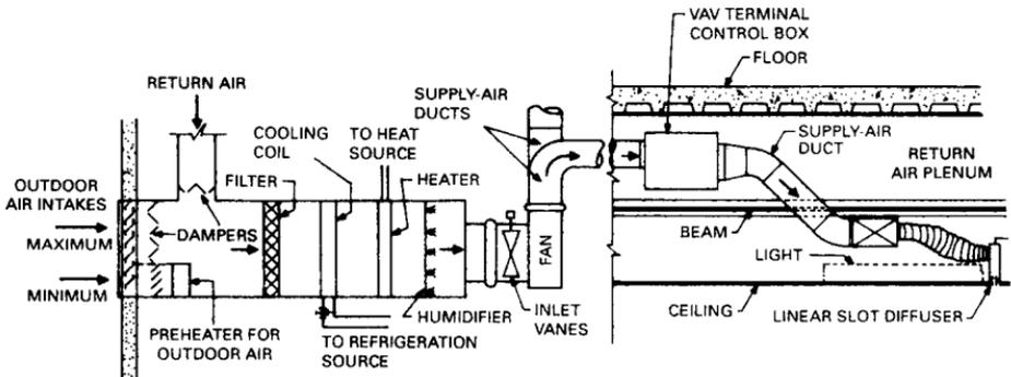
FIGURE 13.38 VAV system varies the supply-air volume to meet changing load conditions.
