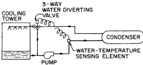
**FIGURE 13.47** Piping layout for control of temperature of water from a cooling tower.
