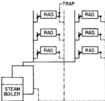
FIGURE 13.15 Wet-return two-pipe steam-heating system.
