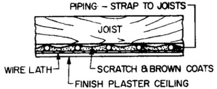
**FIGURE 13.22** Pipe coil embedded above lath and plaster ceiling for radiant heating.
