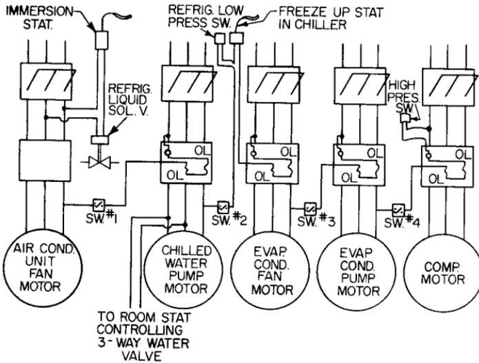
**FIGURE 13.44** Control circuit for a chilled-water system with evaporative condenser.
