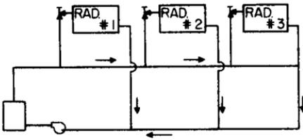
FIGURE 13.6 Two-pipe direct-return hot-water heating system.
