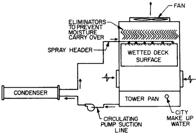
**FIGURE 13.31** Water tower connection to a condenser of an air-conditioning system.
