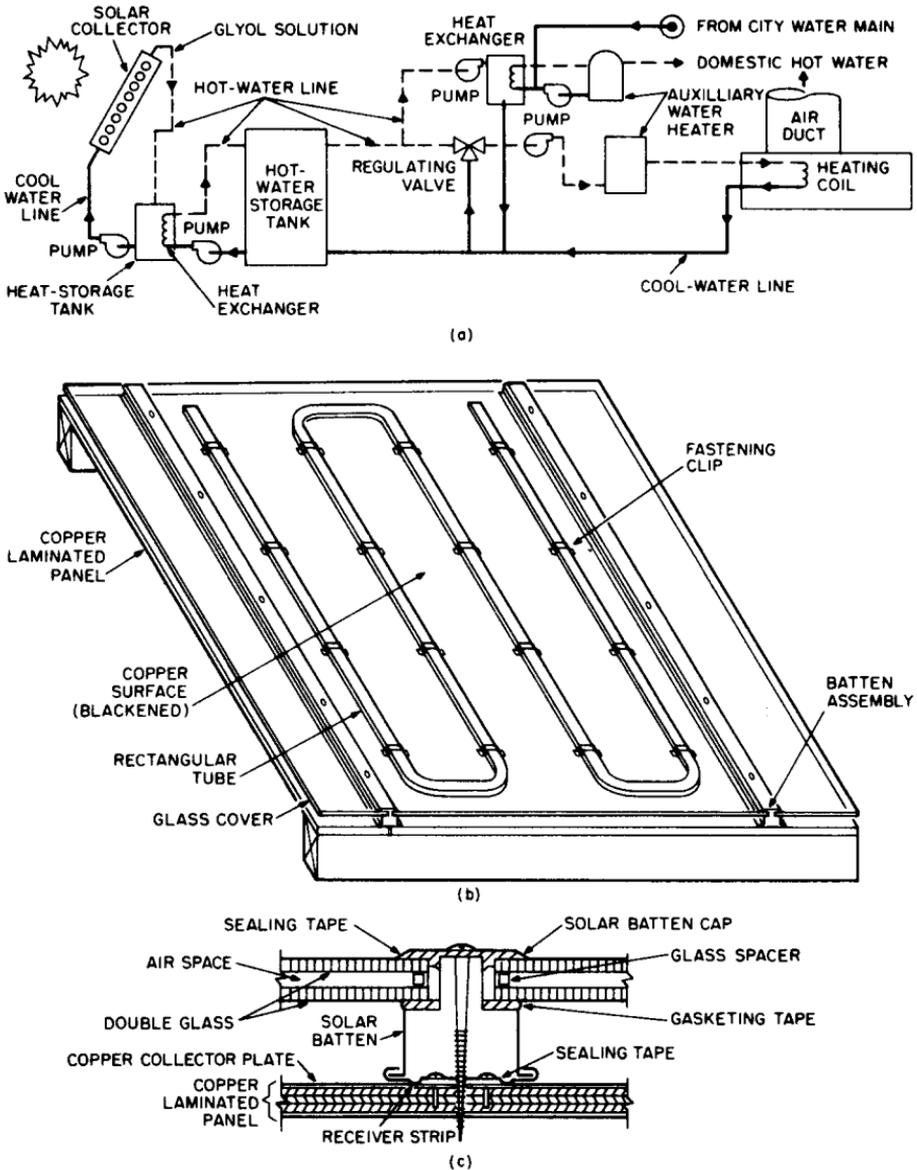
**FIGURE 13.28** Example of a solar-heating system for a building: (a) heat absorbed from solar radiation by a glycol solution is transferred to water for heating a building and producing domestic hot water; (b) solar collector for absorbing solar radiation; (c) detail of the batten assembly of the solar collector. (Reprinted with permission from F. S. Merritt and J. Ambrose, "Building Engineering and Systems Design," 2d ed., Van Nostrand Reinhold Company, New York.)
