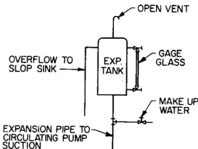
FIGURE 13.9 Open-type expansion tank.
