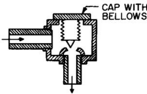
FIGURE 13.14 Drip trap for condensate return of a steam radiator.
