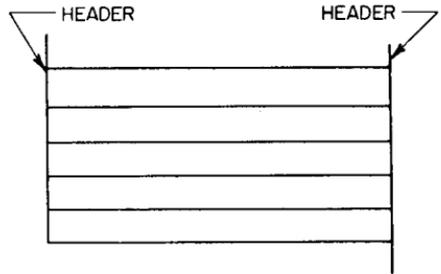
**FIGURE 13.25** Piping arranged in a grid for radiant heating.
