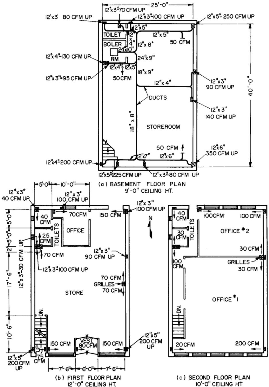
**FIGURE 13.4** Layout of a duct system for warm-air heating of the basement, first floor, and second floor of the building shown in Fig. 13.3. The boiler room is in the basement.
