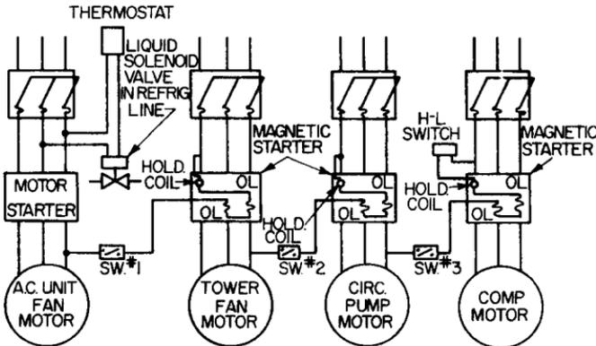
FIGURE 13.43 Control circuit for a cooling-tower-type HVAC system.
