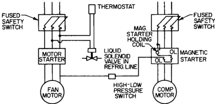
FIGURE 13.41 Pump-down system for control of air conditioning.
