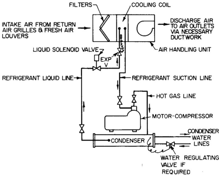
FIGURE 13.29 Direct-expansion air-conditioning cycle.
