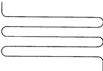
**FIGURE 13.24** Continuous pipe coil for radiant heating.
