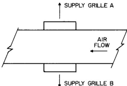
**FIGURE 13.34** Grilles placed back to back on an air-conditioning duct with no provision for adjustment of discharge.
