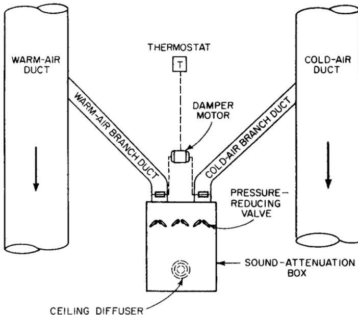
**FIGURE 13.37** Double-duct air-distribution system.
