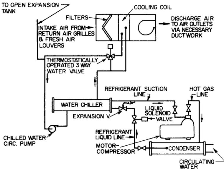
FIGURE 13.30 Chilled-water air-conditioning cycle.
