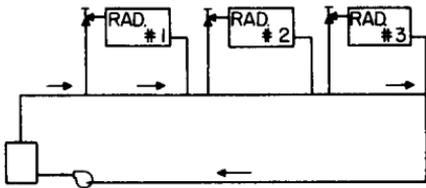
**FIGURE 13.5** One-pipe hot-water heating system.
