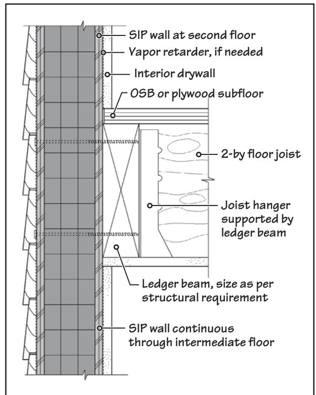
**FIGURE 17.13** Detail at the intersection of a floor and a SIP wall where the SIP wall is continuous through the floor.
