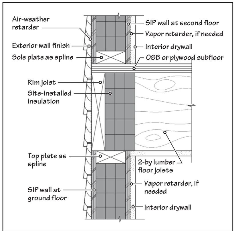
**FIGURE 17.11** Detail at the junction of a SIP floor and a SIP wall. The detail is similar to that used in a conventional wood frame building. Site-installed insulation is needed behind the rim joist.
