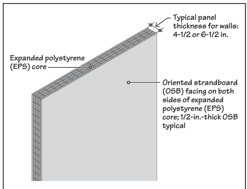
**FIGURE 17.2** Composition of a typical structural insulated panel.
