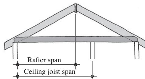
1. The above table applies to a roof live load (or snow load)  $\leq 20$  psf and a light roof cover (such as asphalt shingles). If the snow load exceeds 20 psf and (or) the roof cover is heavier (such as clay or concrete tiles), the span capability of a given rafter size will be smaller.
