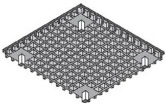
**Two-Way Joist (Waffle) Slab**
