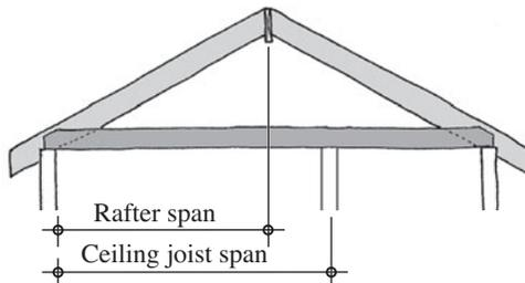
Because the span of a hip or valley rafter is larger than the common rafters, hip or valley rafters are generally one size larger than the common rafters. Thus, for 2 × 8 common rafters, a hip or valley rafter is generally 2 × 10.
